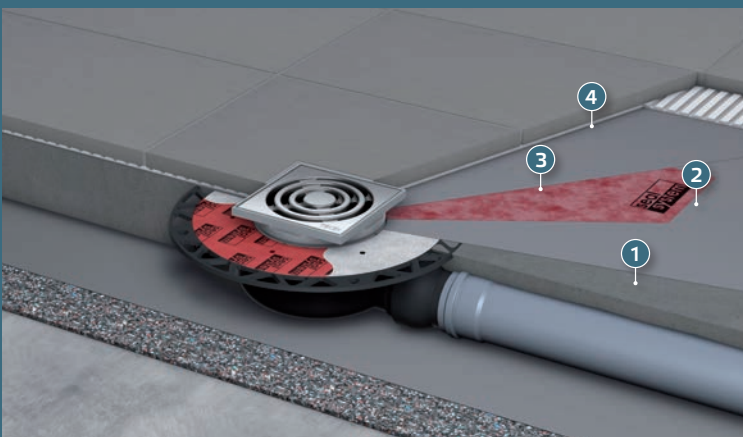
▲ Certified Seal System sealing edge at a shower channel with a point drain on screed (1). The sealing sleeve (3) is laid on the first coat of slurry seal (2), embedded and later overcoated with a second coat (4).
