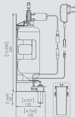
Power supply: Battery box for 6xD batteries
